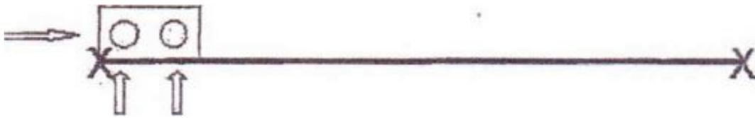
When you level and plumb, always make sure the wooden level fits snugly against the material you are plumbing and the bubble is between the two center lines.
